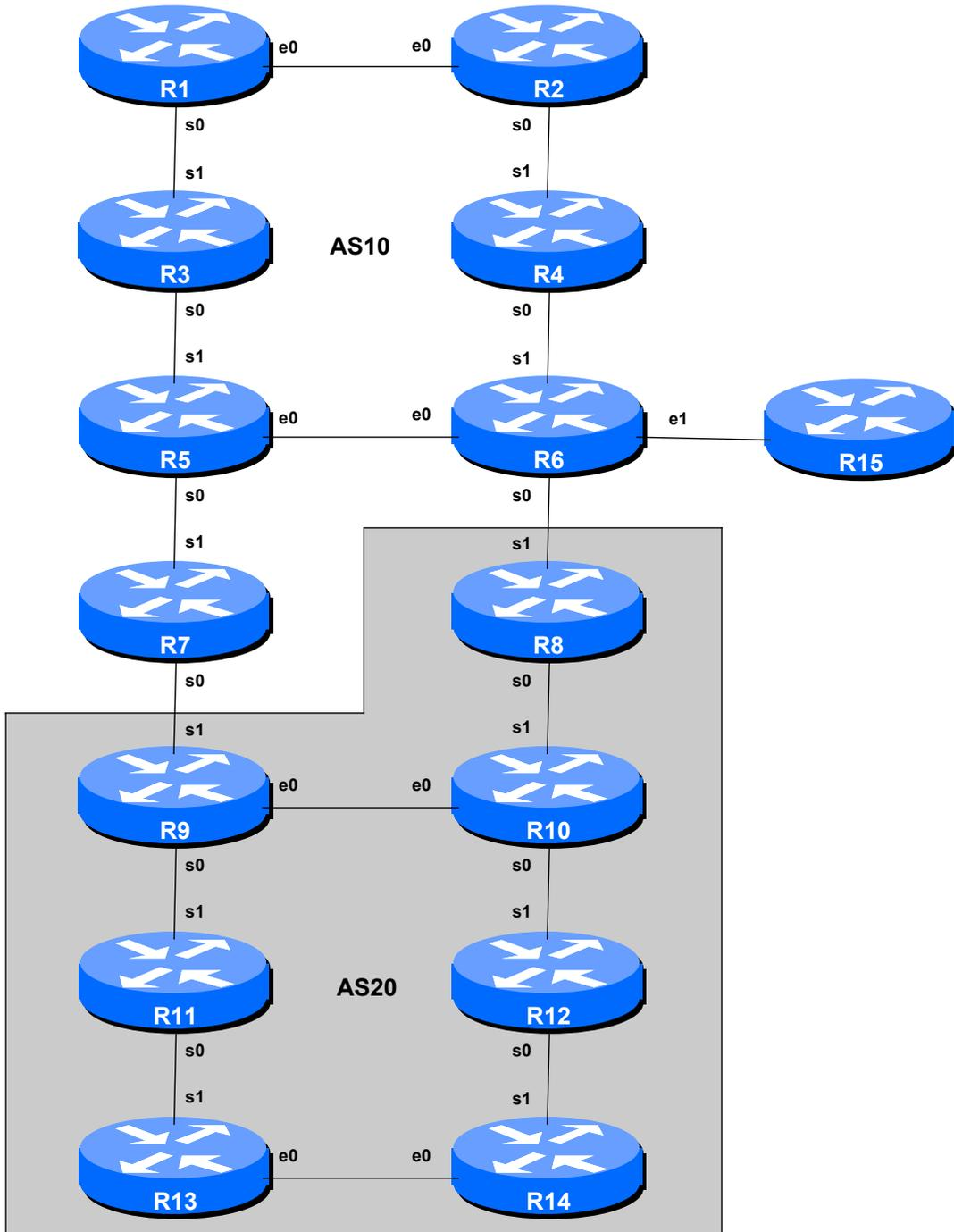
Figure 1 – ISP Lab Basic Configuration
