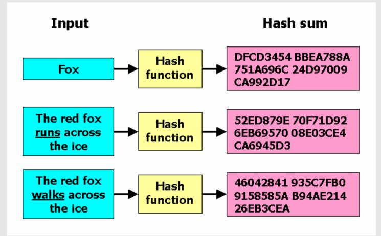
Note the significant change in the hash sum for minor changes in the input. Note that the hash sum is the same length for varying input sizes. This is extremely useful.
